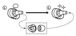
**Note 1:** Change the Long Hybrid silicone rubber earbud and the Fitting supporter to new WF-1000XL (L-ch).
