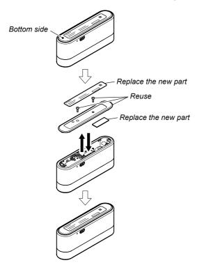
**Note 2:** New WF-1000XL (L-ch) is supplied as a unit of new CRADLE NFC board (with sheet (NFC)) and new model number label together.
