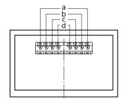
4 Decide the positions of the screws for installing the Base (20) (a).
