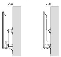
3 Fit Base Adaptor ① by using Screw (PSW 4x10) ② to Base (20) ⓐ when selecting 2-a.
