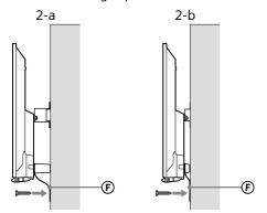
Use a 5 mm diameter screw or equivalent (not supplied).
