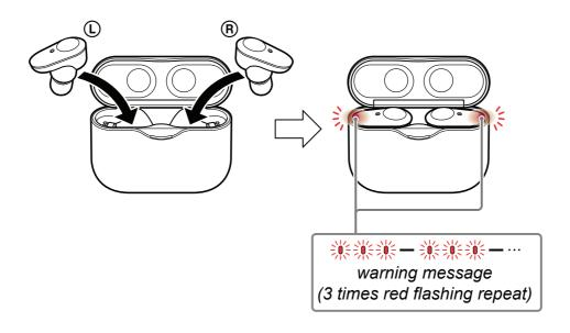
4. Touch and hold the touch sensor control panel on the left and right headset simultaneously, and the indicator changes from warning message (3 times red flashing repeat) to red flashing (slow), in this state release the your finger.
