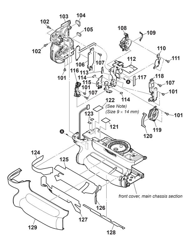
**Note:** When replacing Ref. No. 122, cut the new part to the specific size indicated in the figure before use.
