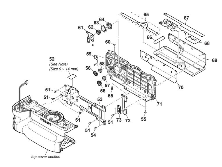
**Note:** When replacing Ref. No. 52, cut the new part to the specific size indicated in the figure before use.
