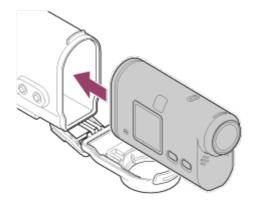
4. Insert the tab of the case body into the slot of the case cover.
