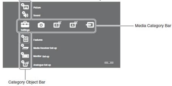
3. Using the volume (left/right) and channel (up/down) Buttons (11 & 12), navigate down the category object bar until you get to Monitor Setup.
